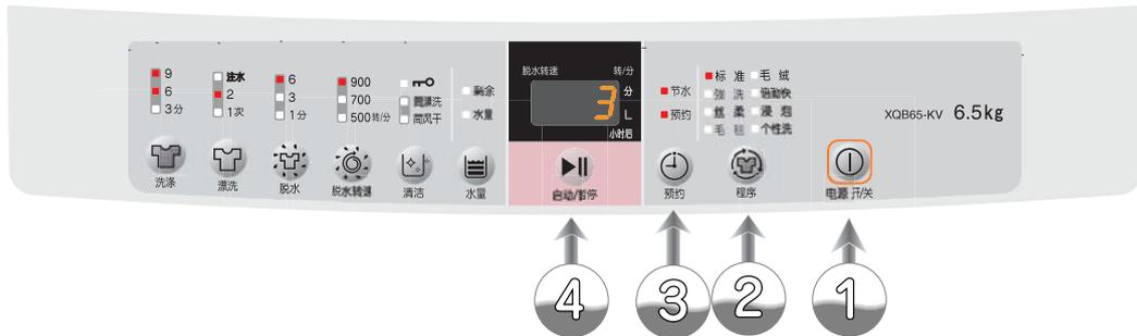
1 放入洗涤物，关闭机盖，按下电源开关按钮
